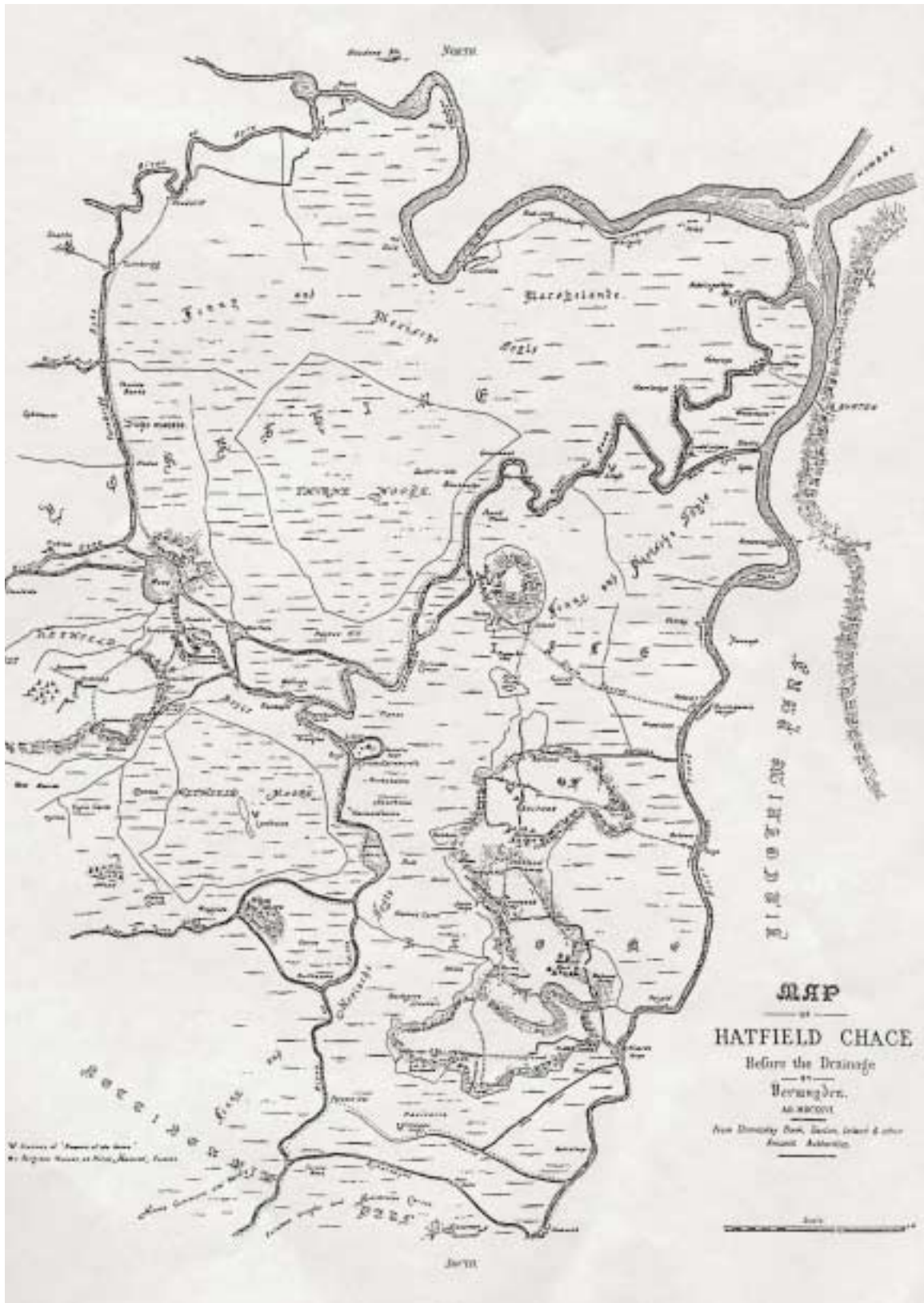
THE ORIGINAL RIVER DON This shows the Don System before Vermuyden's scheme to encourage the whole flow of the River Don down a channel to the River Aire
