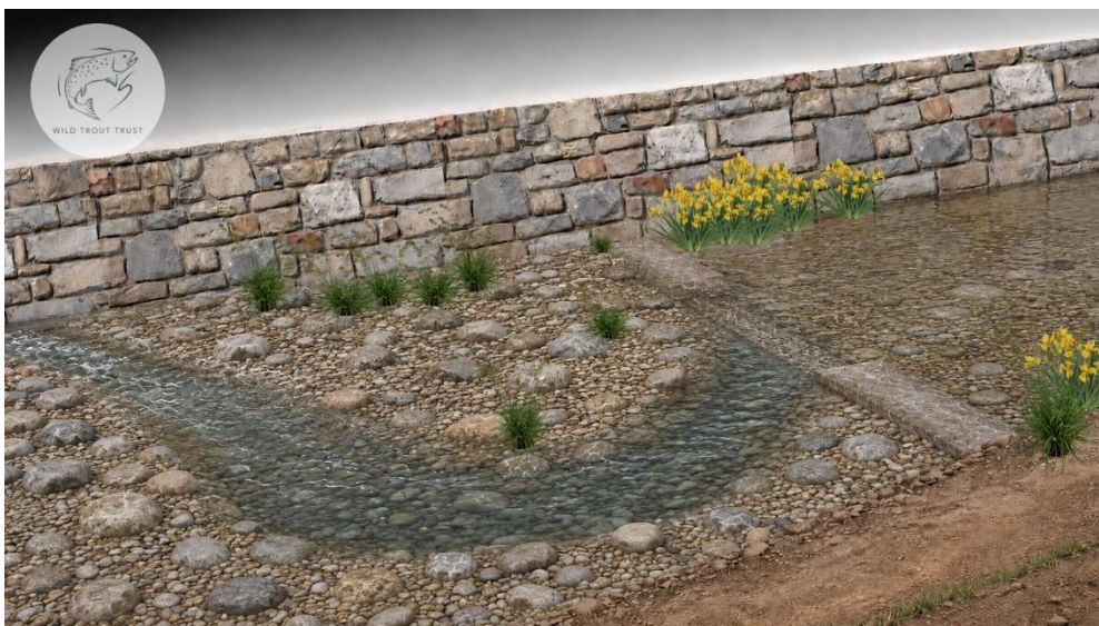
Figure 6: A meandering thalweg (deeper channel carrying most of the flow) concept under low-flow conditions. Perturbation boulder size and placement density must be sufficient to maintain adequate water depth through the slot under low flows. This approach is also likely to produce more ecologically valuable riparian vegetation than the more uniform structures associated with coir roll and pallet installation.
