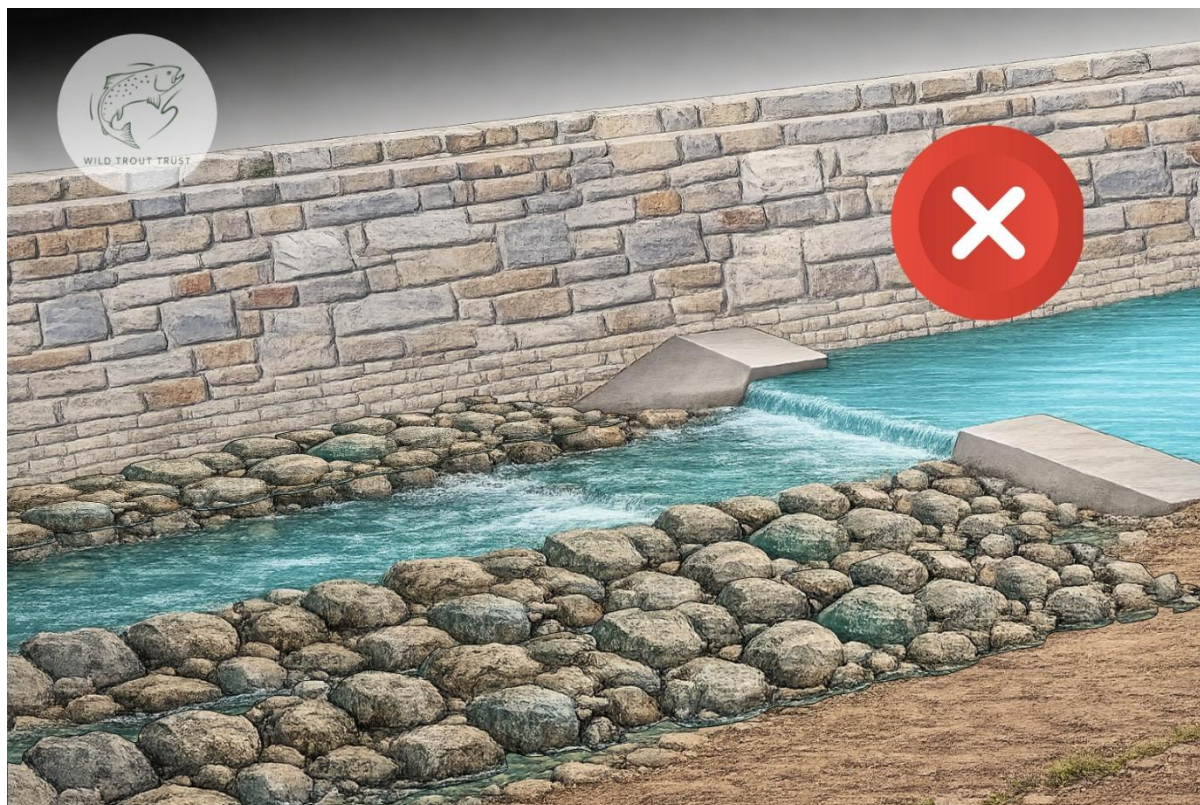
Figure 1: This rock ramp feature fails to address passage at the crest of the structure. It also makes poor use of the available lateral space.
